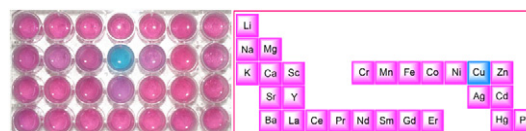
Figure 1. (left) The color changes of SQ1 ( c=10 \mu\text{M} ) in (10 mM) HEPES/THF ( v/v =60/40, pH=7.4) upon addition of 1.0 equiv of various metal ions. From left to right and top to bottom: \text{Li}^+ , \text{Na}^+ , \text{K}^+ , \text{Ca}^{2+} , \text{Mg}^{2+} , \text{Sr}^{2+} , \text{Ba}^{2+} , \text{Fe}^{3+} , \text{Co}^{2+} , \text{Ni}^{2+} , \text{Cu}^{2+} , \text{Zn}^{2+} , \text{Cr}^{3+} , \text{Cd}^{2+} , \text{Mn}^{2+} , \text{Pb}^{2+} , \text{Hg}^{2+} , \text{Ag}^+ , \text{La}^{3+} , \text{Ce}^{3+} , \text{Pr}^{3+} , \text{Nd}^{3+} , \text{Y}^{3+} , \text{Er}^{3+} , \text{Sm}^{3+} , \text{Gd}^{3+} , \text{Sc}^{3+} , blank. (right) Schematic representation of the periodic table of metallic elements.
